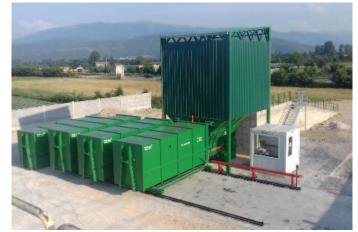
Automatic reloading station type Tehnix - from garbage truck to 32 m³ press-containers
