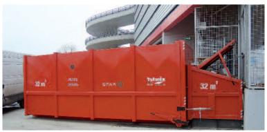
Two-parts rolo press-container 32 m<sup>3</sup> to 10 tons
