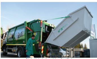
Tehnix skip loader for containers 5 and 7 m<sup>3</sup>
