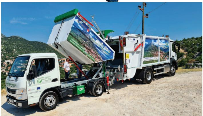
POSSIBILITY OF RELOADING FROM SMALL TO LARGE VEHICLES USING HYDRAULIC EXTENSIONS FOR COMPLETE PRECISION AND ADDITIONAL CLEANLINESS
