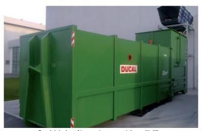
Special desing of two-part press-container with lifter
