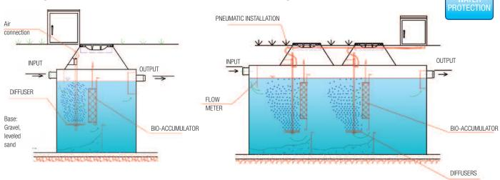
INSTALLATION METHOD: dig a pit, fill up the bottom with gravel, press it manually or with a machine, level and install BIO CESSPIT.
