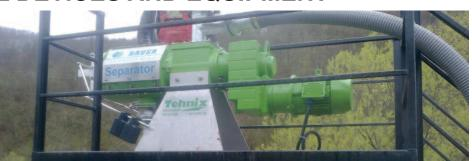
SLUDGE SEPARATOR FOR BIOREACTORS AND FARMS
